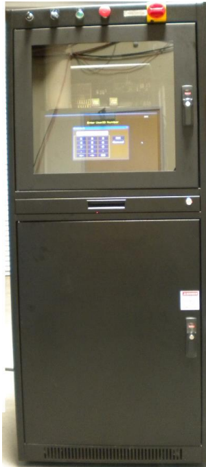
Image 1: Control Unit 24" D x 28" W x 72" H;
